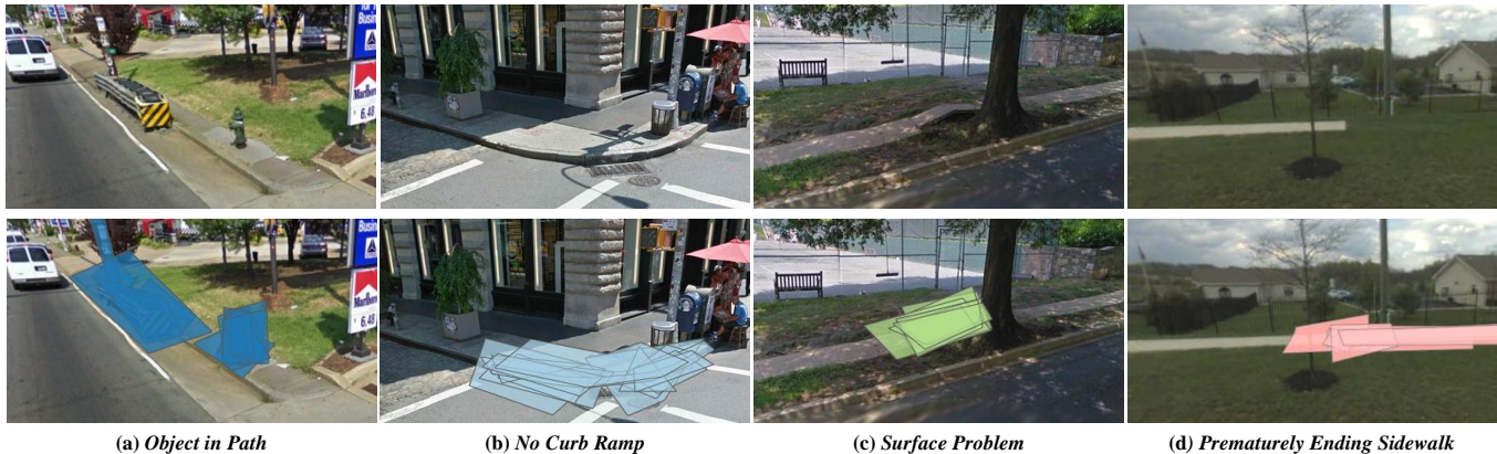
Figure 1: In this paper, we propose and investigate the use of crowdsourcing to find, label, and assess sidewalk accessibility problems in Google Streetview (GSV) imagery. The GSV images and annotations above are from our experiments with Mechanical Turk crowd workers.
